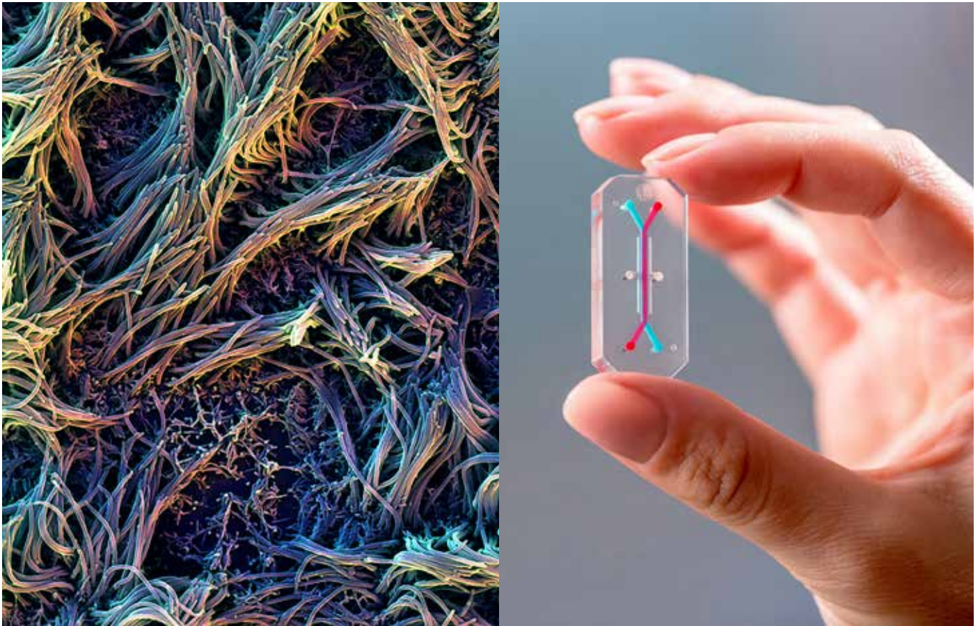
Left: SEM image showing human ciliated cells inside Emulate's Lung-Chip. Donald E. Ingber and Dan Dongeun Huh, 2008. Right: Digital image Emulate's Organ-Chip. Donald E. Ingber and Dan Dongeun Huh. Flexible, clear, silicone polymer, 2008.
